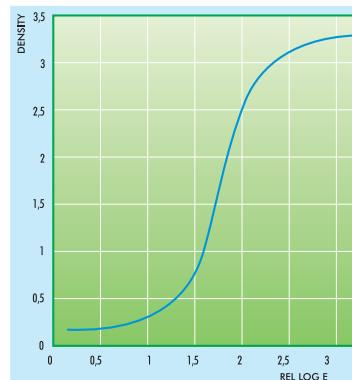
CEA OGA developed in CEAROLL Developer at 35° C (95° F) at 90 seconds processing time
